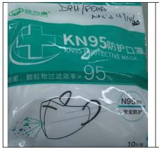
POWECOM Test date – 4/18/20 - Filtration efficiency: 90.6%
